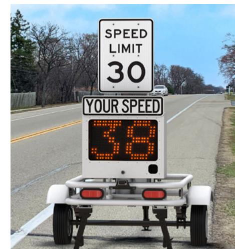
Image of a temporary dynamic speed feedback sign or speed trailer. Source: https://flow.alltrafficsolutions.com
