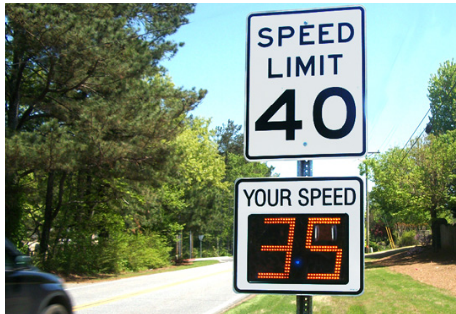
Image of a permanently installed dynamic speed feedback sign. Source: https://www.radarsign.com/
